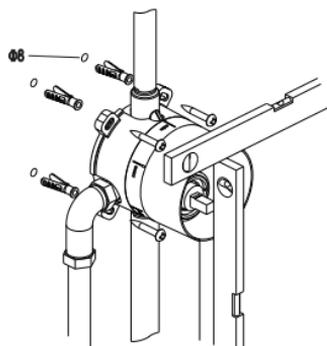
Insert the enclosed plastic cartridges 8 x 40 into the holes and put on the Plastobox sleeve. Level the concealed housing horizontally and vertically, for help use the edges of the sleeve. Finally, firmly tighten with screws 5 x 40 and place on the cover to protect the fitting from damage.
