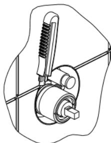
Prior to final assembly first clean off the glue or mortar respectively from the sleeve and the cover, in order to avoid damage to the chrome-plated surfaces. In the next step, cut along the ceramics the excess part of the sleeve using knife. Take care not to damage the chrome-plated parts with the blade.
