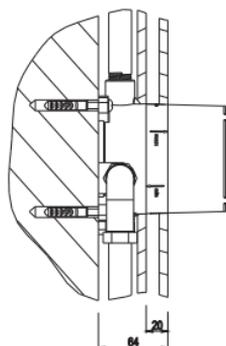
Pay special attention to the max and min marks on the sleeve label. When mounting it is necessary to envisage the top ceramic layer, which must lie within the tolerance range of the label. The tolerance range is 20 mm.
